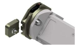
Step 3. Install the *tool part holders* and place the *tool part* and *end-effector* assemblies in the *tool part holders* to make sure that there is space as appropriate. The *tool part holders* must be installed as instructed in the *user guide*. (*User guide chapter: 6.6*)
