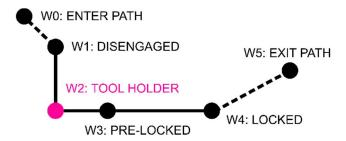
Waypoint W2 is the reference point for the other waypoints, so program/teach waypoint W2 first and from there move the cobot linear in the axial direction to program/teach W1 and from W2 in the radial direction to teach/program W4 (and W3). Waypoint W4 can be programmed/teached with a slight incline to lift the *tool part* free of the *tool part holder*.
