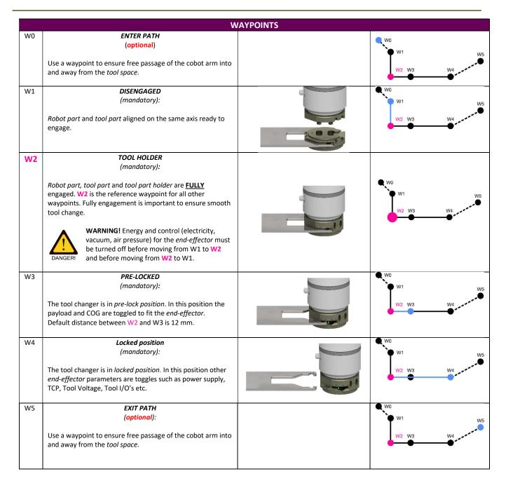
Step 2. After testing that tool changes executes correctly, re-install the pass-through modules, cables and hoses to provide connectivity to the *end-effectors*. Then setup the cobot to toggle parameters like voltage, pneumatic and vacuum OFF before tool change takes place and ON after tool change has taken place. You should toggle these parameters in waypoint W4 or W5.
