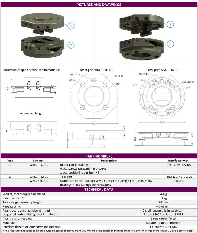
\* The rated payload is based on the payload's center of gravity being 100 mm from the center of the tool changer, a dynamic force of maximum 2G and of 5. Maximum allowed payload must always be calculated for the application.
